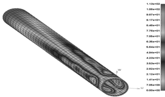
Fig. 8. The wall stress in the blood vessel model for early flow deceleration t=0.4 s; Rigid walls [Pa]
