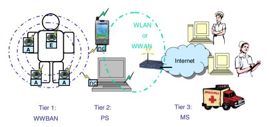
Fig. 1. WWBAN integrated into a telemedical system for health monitoring.
