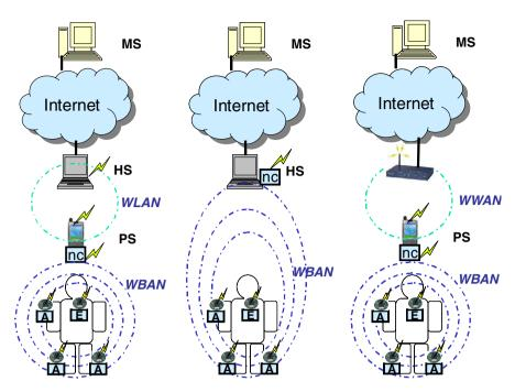
Fig. 2. WWBAN deployment scenarios. Legend: A, activity sensor; E, heart sensor; WBAN, wireless body area network, PS, personal server; WLAN, wireless local area network; WAN, wide area network; HS, home server; MS, medical server; nc, WBAN network coordinator.
