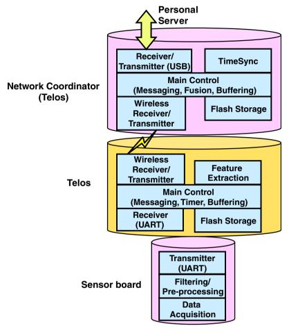
Fig. 6. WBAN software architecture.
