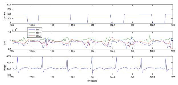
Fig. 3. ECG, acceleration, and foot switch data collected by the WWBAN prototype during normal walking.
