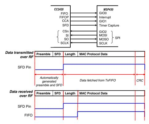
Fig. 7. Interfacing CC2420 RF transceiver (top). IEEE 802.15.4 frame format and pin activity (bottom).
