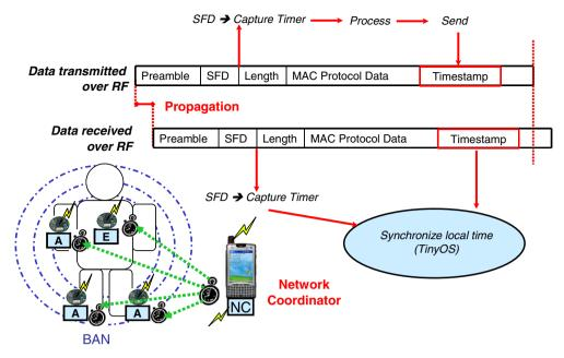
Fig. 8. Time synchronization in WBAN prototype.
