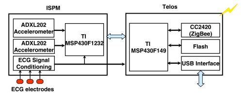
Fig. 5. Block diagram of an ActiS sensor node.
