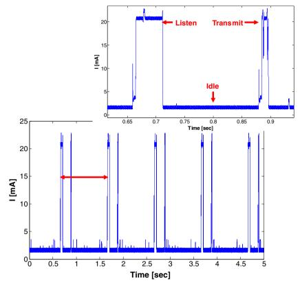
Fig. 10. Actis current consumption during 5 s of operation. Red arrow marks one super frame cycle. (For interpretation of the references to color in this figure legend, the reader is referred to the web version of this paper.)
