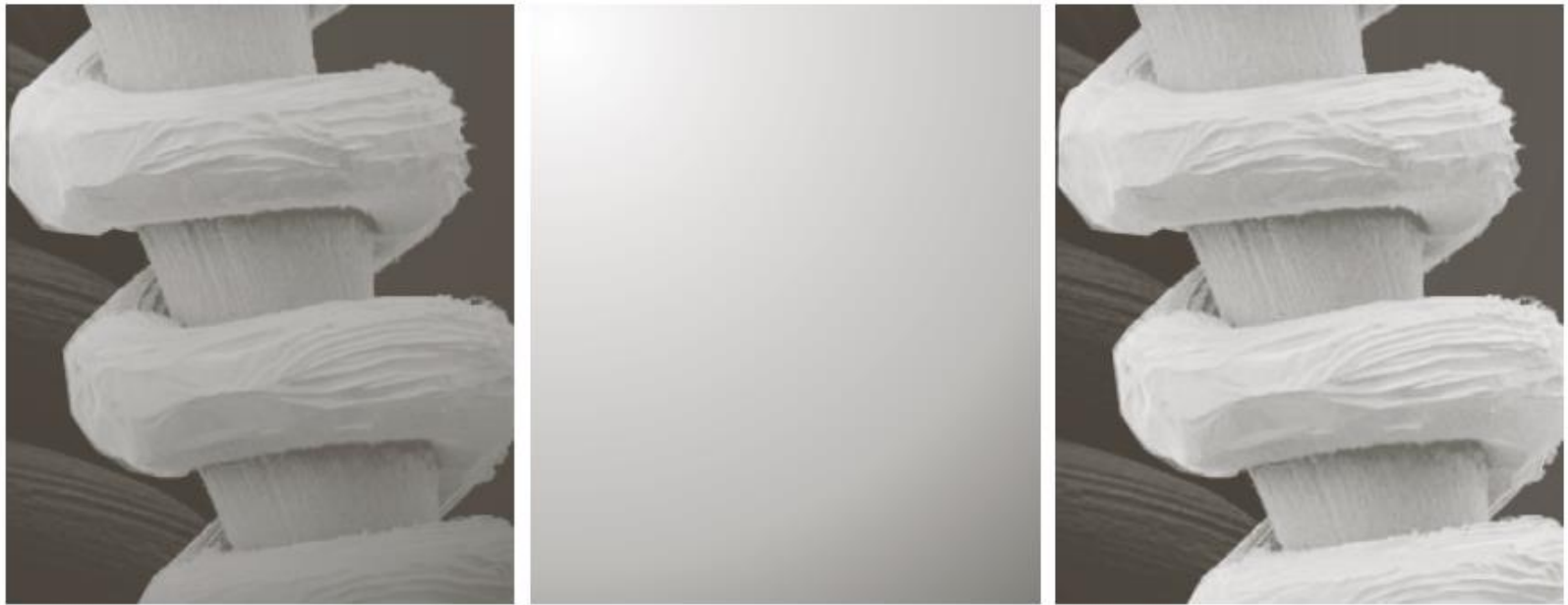
FIGURE 2.29 Shading correction. (a) Shaded SEM image of a tungsten filament and support, magnified approximately 130 times. (b) The shading pattern. (c) Product of (a) by the reciprocal of (b). (Original image courtesy of Mr. Michael Shaffer, Department of Geological Sciences, University of Oregon, Eugene.)
