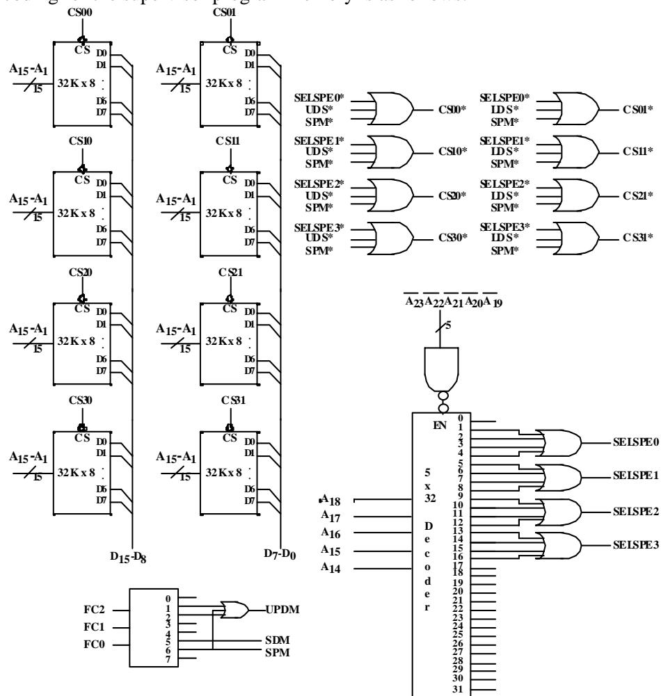
The address decoding for the user program and data memory is as follows
