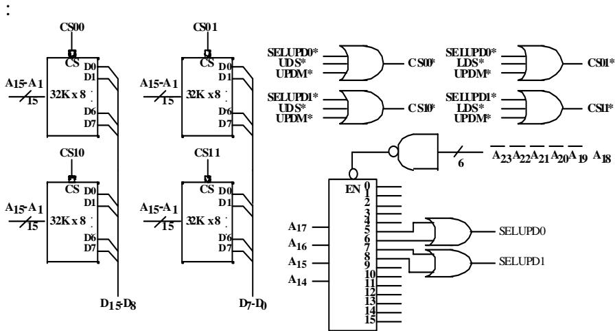
The address decoding for the supervisor data memory is as follows:
