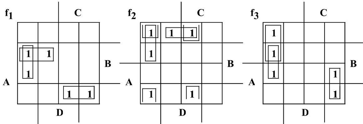
$$f_1 = \overline{B}\overline{C}\overline{D} + \overline{A}\overline{B}\overline{C} + \overline{A}\overline{B}\overline{C}$$
