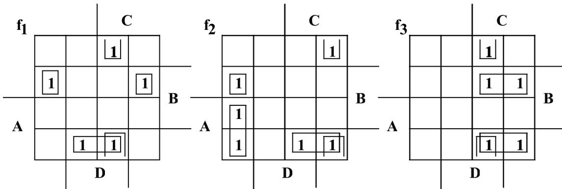
$$f_1 = \overline{B}\overline{C}\overline{D} + \overline{A}\overline{B}\overline{C}\overline{D} + \overline{A}\overline{B}\overline{D} + \overline{A}\overline{B}\overline{C}\overline{D}$$
