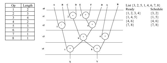
6. (10 points) For the data lifetime chart shown, use the left edge algorithm to obtain an efficient register allocation.
