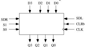
Write a VHDL description of an 8-bit bi-directional shift register that uses two 74194s as components. The parallel inputs and outputs to the 8-bit register are X and Y. The serial inputs are RSD and LSD.
