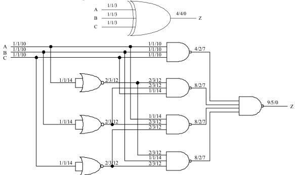
2.2 Use the rules given in Tables 2.3 and 2.4 to calculate the probability-based testability measures for a three-input XNOR gate and for its NAND-NOR implementation. Assume that the probability-based controllability values at all primary inputs and the probability-based observability values at all the primary outputs are 0.5 and 1, respectively.
