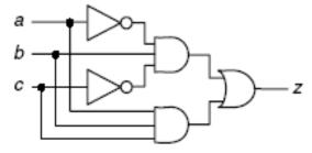
There are 14 nodes in the circuit. Thus, there are  $14 \times 2 = 28$  single stuck-at faults. For multiple stuck-at fault, it has  $(2 + 1)^{14} - 1 = 4782968$  multiple stuck-at faults. For collapsed single stuck-at fault:
