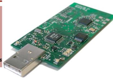
Designed at the University of California, Berkeley, by TinyOS integration between the hardware and the TinyOS operating system. TinyOS is a small, open-source, component-based operating system also developed at UC Berkeley. TinyOS was specifically designed to support the networked sensor regime. By leveraging their intimate knowledge of both the hardware and TinyOS layers, Moteiv can promise the highest levels of support to their customers.
