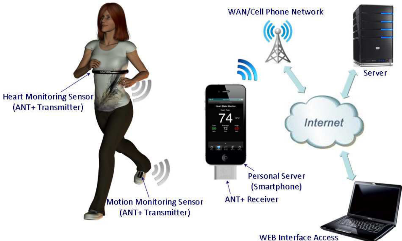
Fig. 1. System organization of the monitoring system
