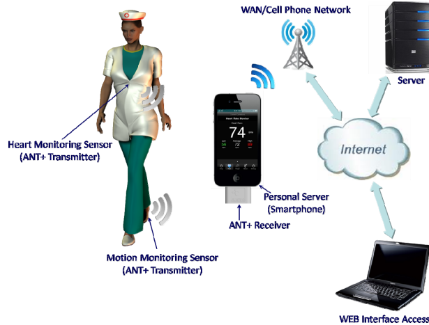
Fig. 1. Real-time monitoring of occupational stress using Wireless Body Area Network of wearable sensors.
