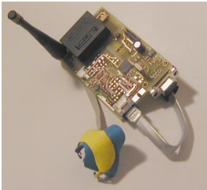
Figure 2. Wireless Intelligent Breathing Telemetry sensor (WIBRATE)
