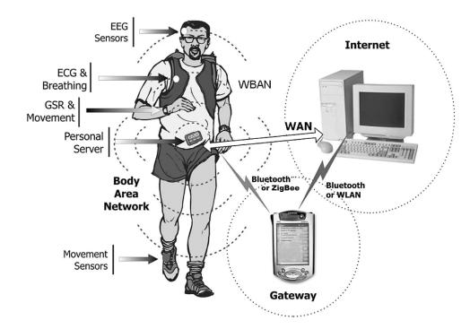
Fig. 3. Typical system architecture of m-health monitoring systems [2].
