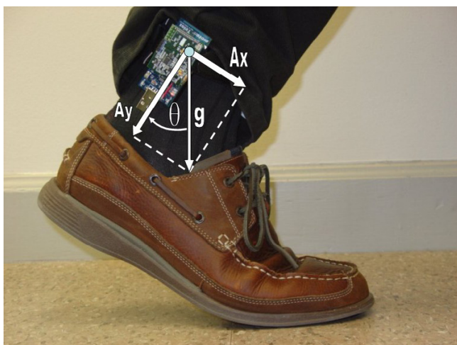
Figure 5 Activity sensor on an ankle with symbolic representation of acceleration components
