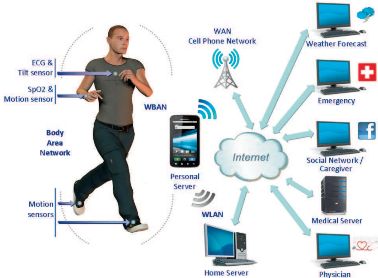
FIGURE 1. SYSTEM ARCHITECTURE OF THE UBIQUITOUS HEALTH MONITORING SYSTEM
