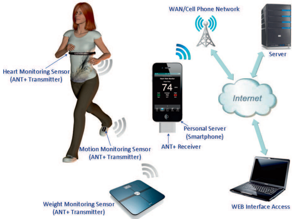
FIGURE 3. SYSTEM ARCHITECTURE OF THE UAHEALTH
