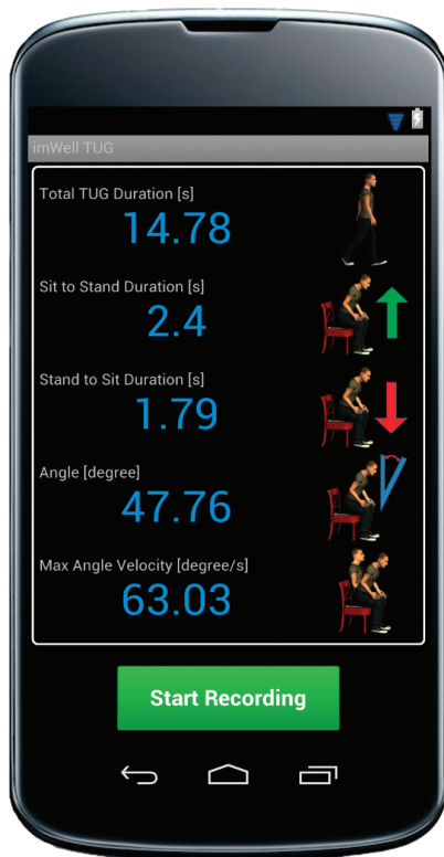
Figure 4. sTUG: Smartphone TUG Android application screen displaying the parameters of the TUG test.
