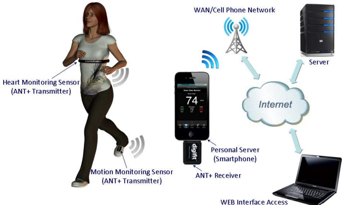
Fig. 1. System organization of the monitoring system
