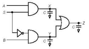
**c.** (10 points) Compute the switching power consumed by the multiplexer, assuming that all significant capacitances have been lumped into the three capacitors shown in the figure, where C = 0.3 pF. Assume that VDD = 2.5 V and independent, identically-distributed uniform white noise inputs, with events occuring at a frequency of 100 MHz. Perform this calculation for the following: (i) a static, fully-complementary CMOS implementation, (ii) a dynamic CMOS implementation.
