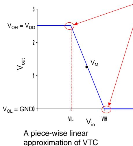
By definition,  $V_{IH}$  and  $V_{IL}$  are where  $dV_{out}/dV_{in} = -1$  (= gain)
