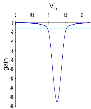
Gain is a strong function of the slopes of the currents in the saturation region, for  $V_{in} = V_M$
