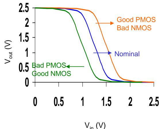
process variations (mostly) cause a shift in the switching threshold
