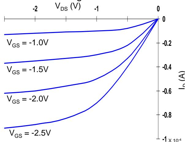
PMOS transistor,  $0.25\mu m$ ,  $L_d = 0.25\mu m$ ,  $W/L = 1.5$ ,  $V_{DD} = 2.5V$ ,  $V_T = -0.4V$
