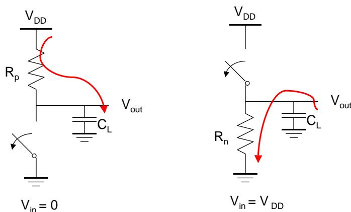
Gate response time is determined by the time to charge  $C_L$  through  $R_p$  (discharge  $C_L$  through  $R_n$ )
